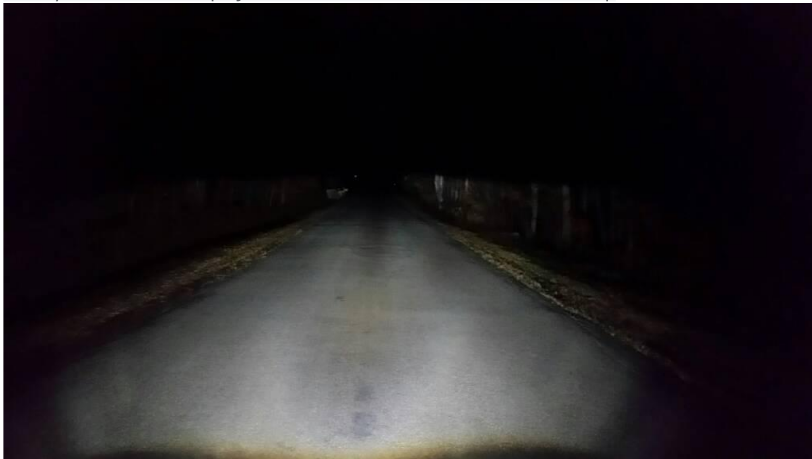
Factory 2015 GMC Sierra projector with 35 watt 5000k Morimoto HID setup
