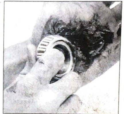
34.15 Work grease into the bearing rollers by pressing it against the palm of your hand
