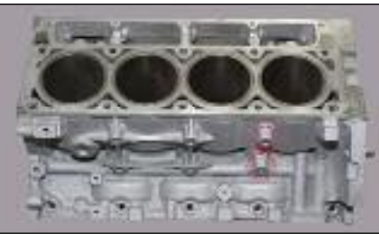
The Gen IV aluminum blocks have two extra bolt holes on the driver's side.
