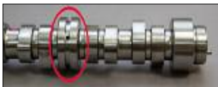
The second journal was grooved and had a hole that fed oil into the hollow core for the engines with VVT.
