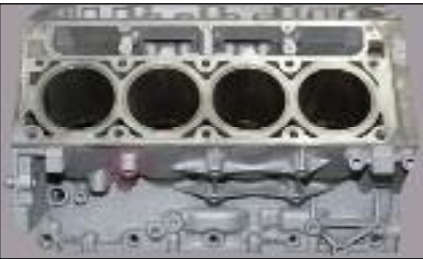
The Gen IV aluminum blocks have one extra bolt hole on the passenger side.
