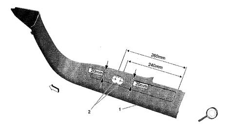
**Note:** Always check scale, size and position of all holes before drilling. Failing to do so may cause damage to the vehicle, misalignment of components or the inability to install the accessory.
