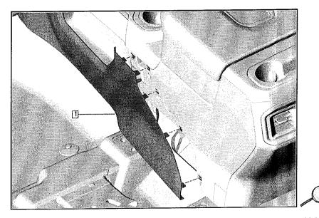
8.3. Starting from the rear, use a flat bladed plastic trim tool to aid in the removal of the panel (1) from the front floor console.
