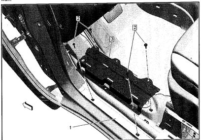
6. Remove the harness sill protector (3) from rocker panel (1).
