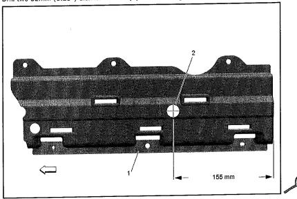
15. Drill a 19 mm (3/4") hole (2) into the harness sill protector (1) according to the dimensions shown.
