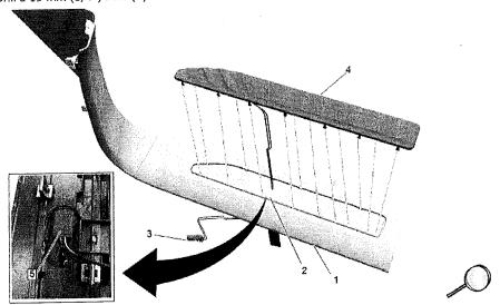
Note: It is important for the circuit board (5) to fit in the holes (2).
