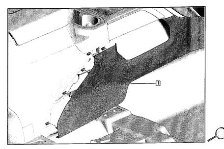
8.5. **Right Front Floor Console Extension Panel:** Starting from the rear, use a flat bladed plastic trim tool to aid in the removal of the front floor console extension panel (1) from the front floor console.
