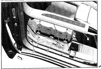
27. Insert the electrical connector (6) of the illuminated sill garnish molding (1) through the previously drilled hole (4) in the harness sill © 2022 General Motors. All rights reserved.
