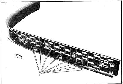
12. Disengage the sill center tabs (1) on the back side of the sill garnish molding.
