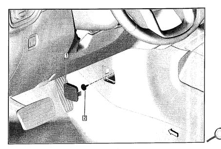
8.1. **Left Front Floor Console Extension Panel:** Front Floor Console Extension Panel Bolt Access Hole Cover (1) » Remove 8.2. Front Floor Console Extension Bolt (2) » Remove Upon reassembly tighten the bolt to 2.5 N.m (22 lb in).
