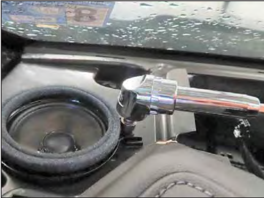
5. Remove two (2) 7mm screws securing speaker to dash, disconnect harness and remove speaker.
