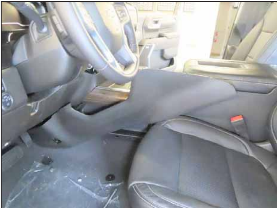
7. Pry off center console lower side panel on driver's side to release ten (10) clips and remove panel.
