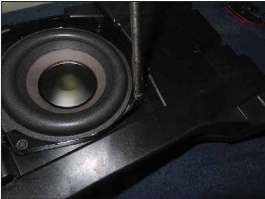
17. Remove four (4) 1/4" screws securing subwoofer to enclosure, disconnect harness and remove subwoofer.
