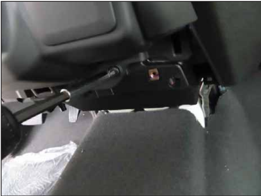
5. Remove two (2) Torx T15 screws exposed by removal of lower center stack panel.
