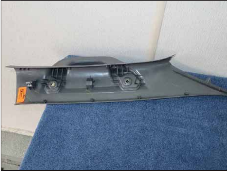
2. Pry out top of pillar trim panel to release one (1) clip, then pull panel up to remove.
