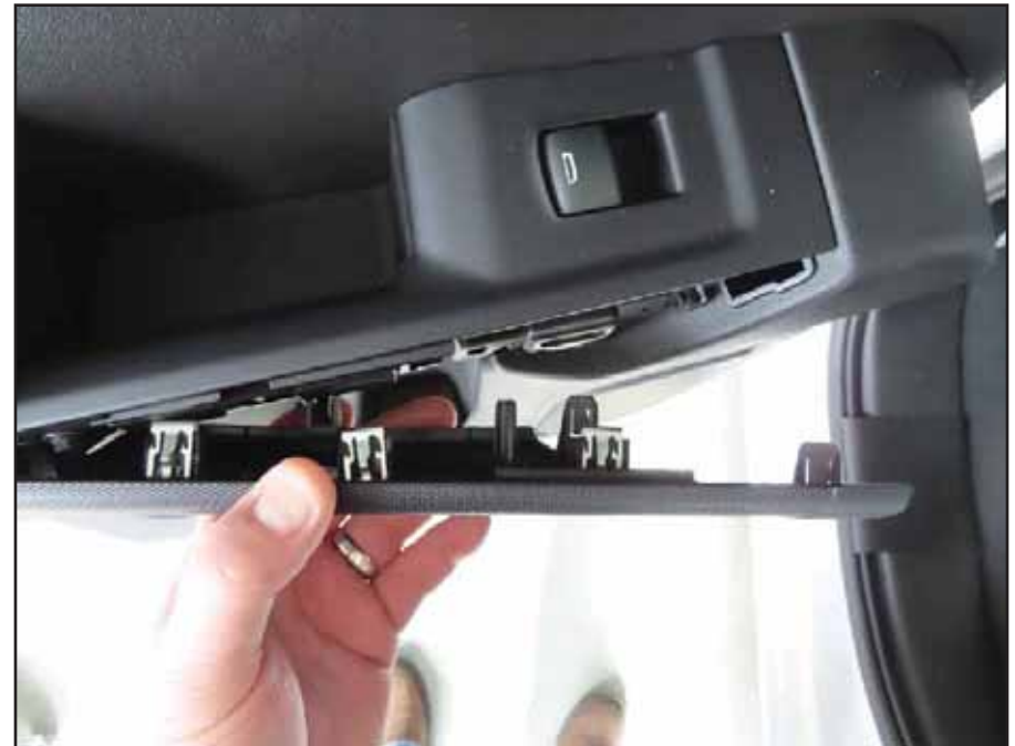
2. Starting at front/lower corner, pry off door pull handle outer cover to release six (6) clips and remove.
