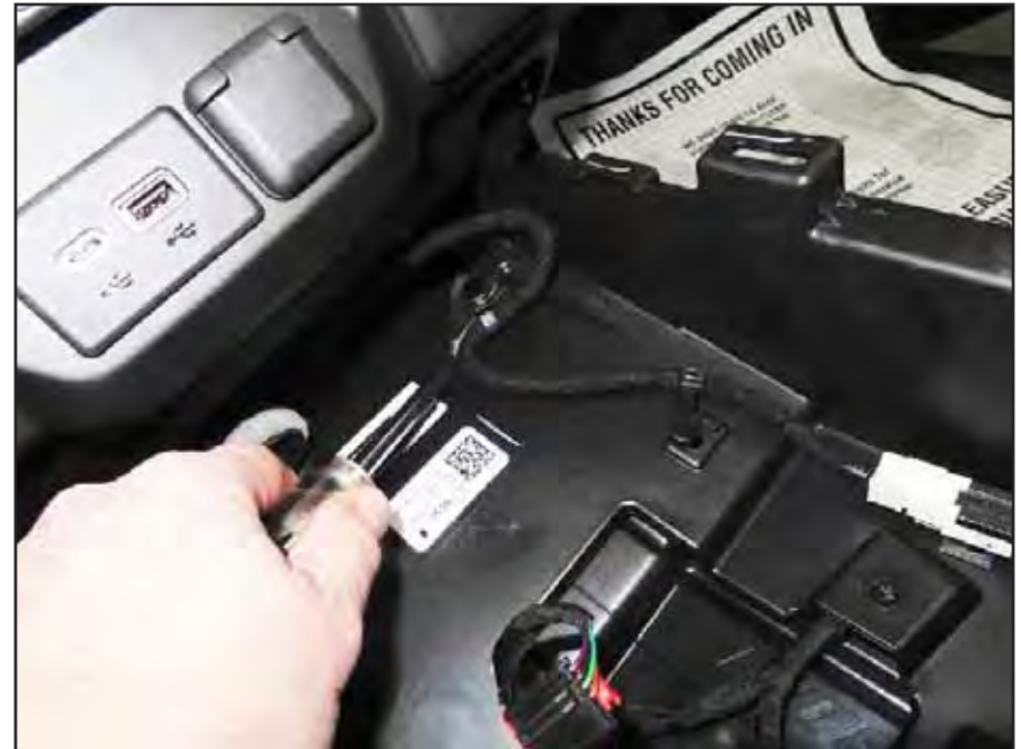
10. Pry up rear cupholder trim panel to release four (4) clips and remove trim panel.
