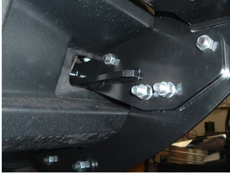
Figure 7. Mounting Side Member.
