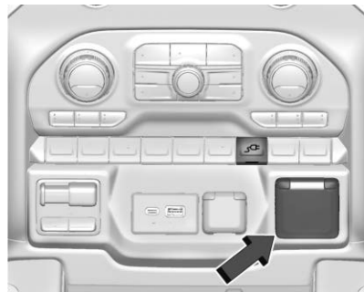
In Cab Power Outlet and DC/AC Switch
