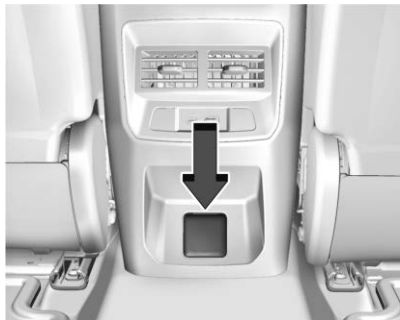
Rear of the Center Console Outlet
