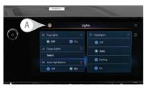
► To enable the IntelliBeam system, which automatically turns the high-beam headlamps on/off based on traffic conditions at night, go to Controls > Lights > Auto High Beams. The exterior lamps must be in the Auto setting. A white ♠ on the instrument cluster indicates the system is on. A blue ♠ appears when the high-beam headlamps are on.
